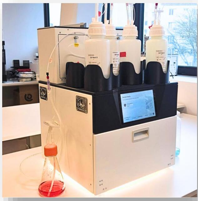
**GenSampler®** - 24/7 fully automated fermenter and bioreactor sampler, up to 24 vessels, plug and play and compatible with all kind of vessels
